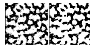
Figure 5 presents the control image sample (left) and the same sample after Erode filter followed by Dilate were applied (right).
