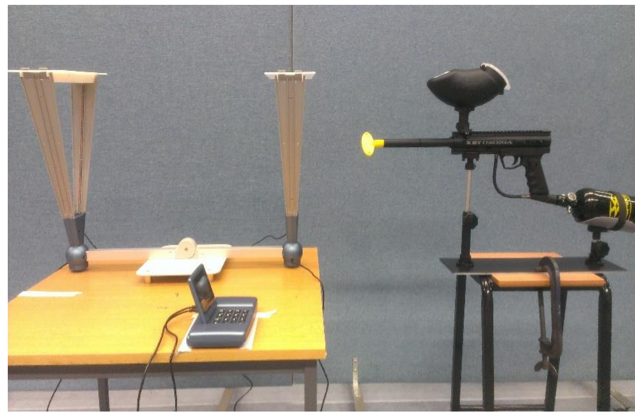
Figure 1. Experimental set-up of the marker and chronograph
